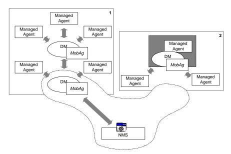
Figure 5 – Mobile Disman Architecture.
