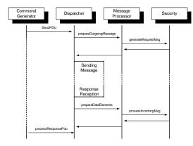
Fig. 1. Commands flow inside an SNMP Entity.
